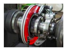
The MAGMA engineering team tests each friction formula and brake disc to analyze real-time noise, vibration, and harshness (NVH) data. This information supports the continuous improvement process, driving product evolution.
